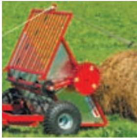
The Buggy tips back easily to self-load the bale
