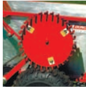
To engage the drive wheel simply drop it down onto the tyre
