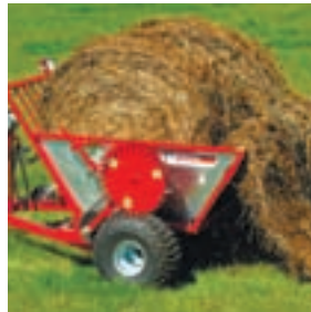
The Buggy tips back easily to self-load the bale
