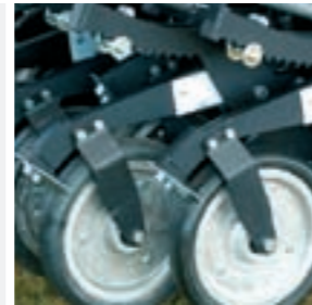
New style press wheels with finer height settings
