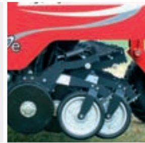
New style press wheels with finer height settings
